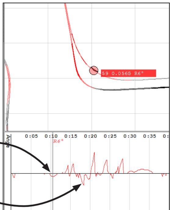
If your angle shows a similar graph pattern in R4 as below, the sensor is installed in a wrong direction. Make sure the arrows on the sensor case is pointed to the front of the bike.
