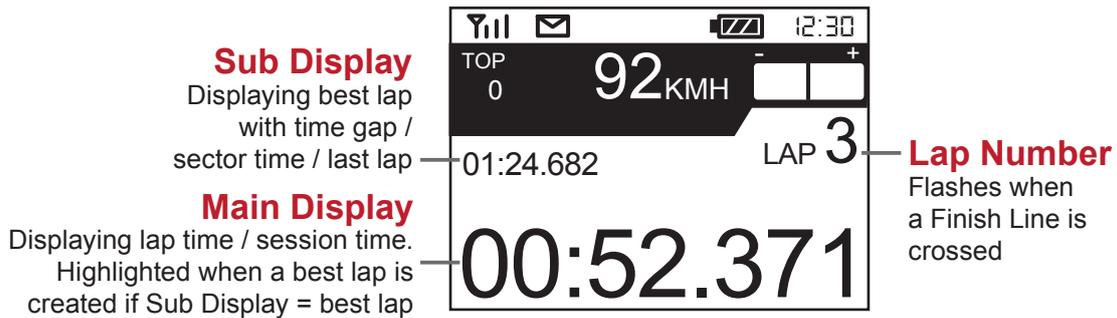
The upper half is the same as Drive mode, displaying top speed, current speed, and longitudinal G. Angles are not displayed. The lower half consists of three components: Main Display, Sub Display, and Lap number.
