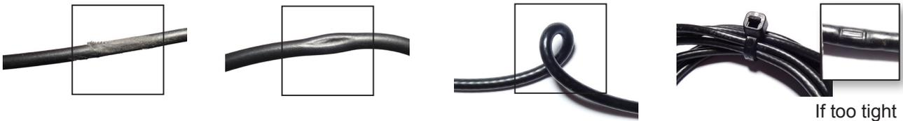
Examples of damaged antenna cable
