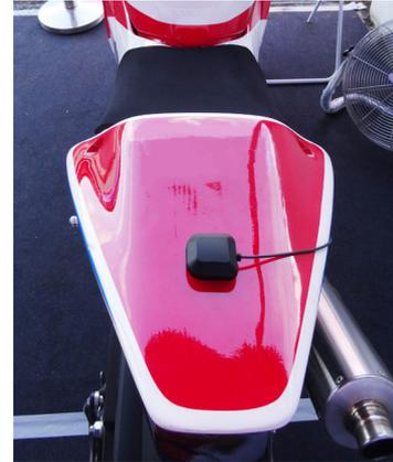
To install, please use the supplied Dual Lock tape to adhere the GPS antenna to a location with a clear view of the sky. To avoid signal loss, the cable run must not be kinked or crushed, or have a bend diameter less than 2 inch (5 cm). The cable should be laid as straight as possible.
