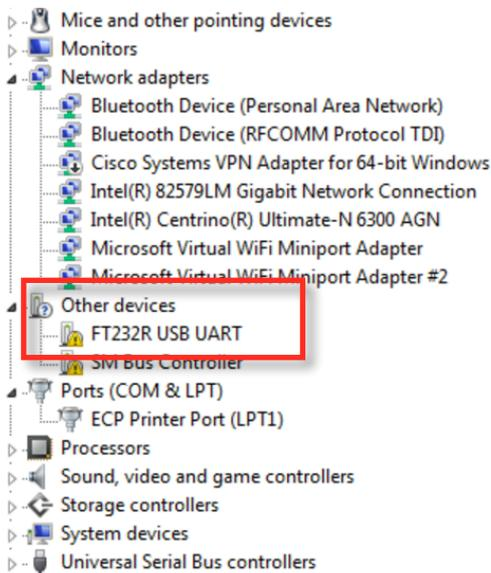
1. Right click on the FT232R device in the device manager, and select UNINSTALL in the menu to uninstall the device.
