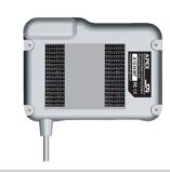
APEX timer mount uses 3M Dual Lock 400 strips and 250 pads, which is the strongest bonding combination of the Dual Lock system. DO NOT replace the 400 strips with 250 strips or pads.
