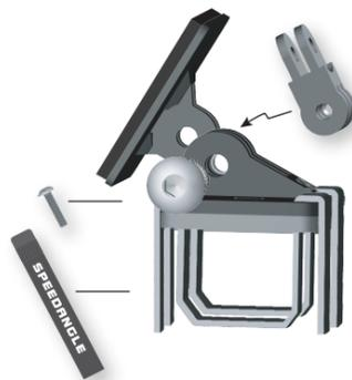
2. Adhere the two 3M Dual Lock 400 strips to the back of APEX.
