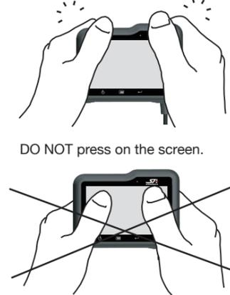
4. To remove APEX from the mount, wrap your fingers around its upper front. Use your thumb base as a pivot and prise the upper end up.
